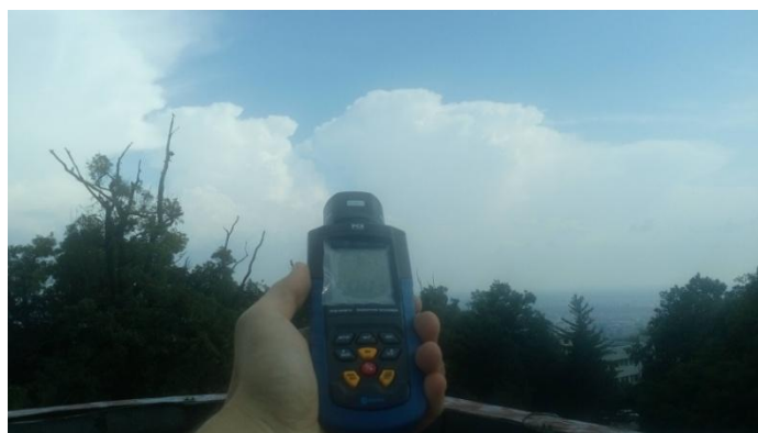
Fig.1 Measurement of gamma ray radiation increase in approaching storm.
